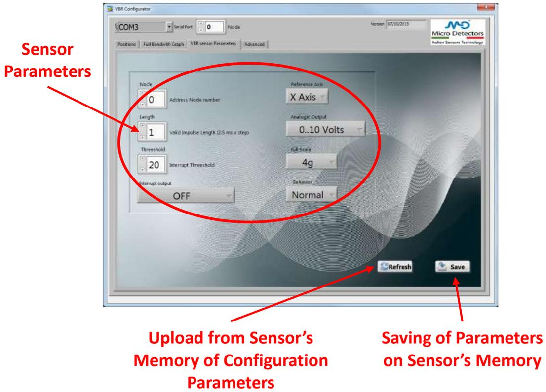
TAB 4: Direct command serial configuration.
