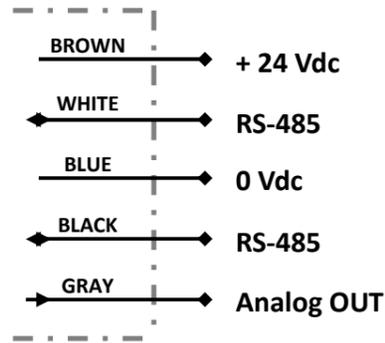
(The type of analogue output can be programmed through the RS-485 Bus)
