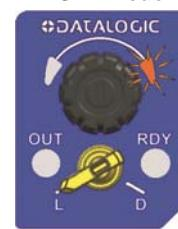
Rotate the sensitivity adjustment knob in counterclockwise direction until OUT LED turns ON.
