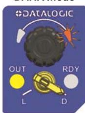
Rotate the sensitivity adjustment knob in clockwise direction.
