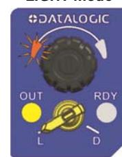
Rotate the sensitivity adjustment knob in counterclockwise direction.
