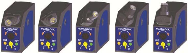
The operating distance is measured starting from the lens front face. The reading direction can be changed inverting the cap and lens.
