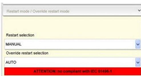
Figure 42 - ACM Configuration: Auto Override Restart Selection
