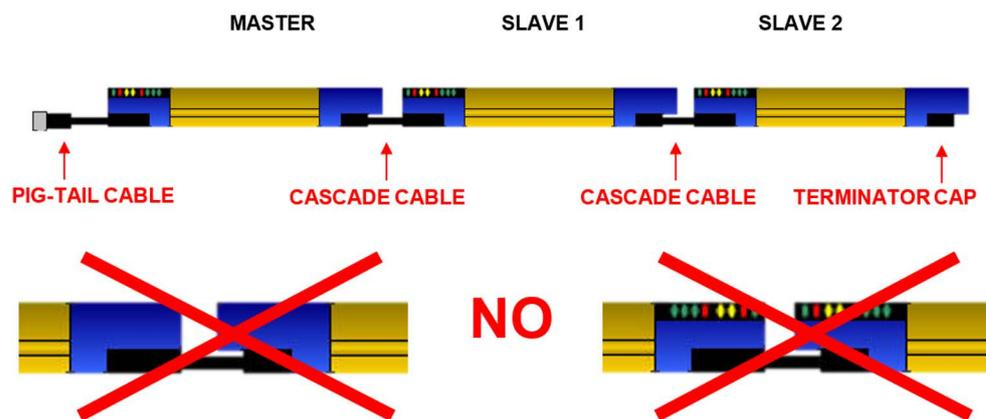
The Cascade connection can be done by using two or three Light Curtains (Standard Model), which can have different length and resolution.
