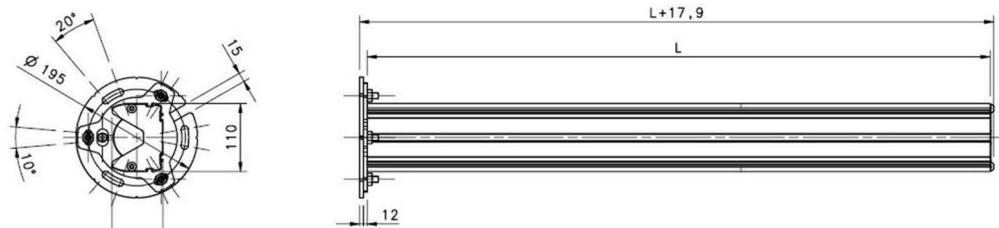
Figure 12 - Dimensions (mm)
