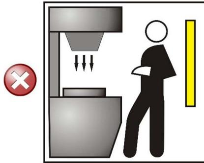
Figure 3 - Wrong light curtain positioning
