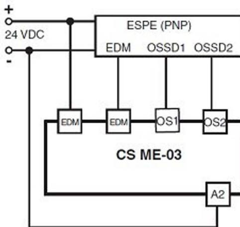
Figure 32 - EDM relay
