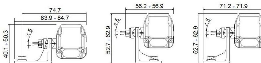
Figure 8 - Angled fixing bracket + Orientable support
