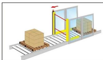
**Figure 16 - L-shaped version with integrated Muting sensors for unidirectional Muting**
