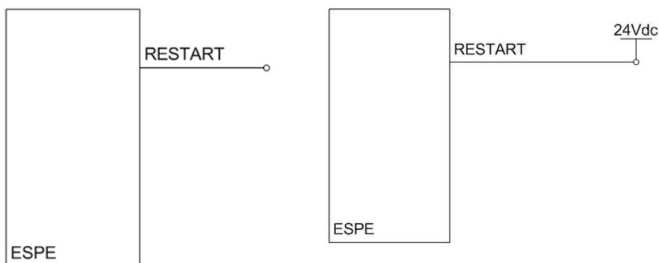
**Manual Restart:** after the ESPE has detected an opaque object in the controlled area, the light curtain begins its normal functioning only by pressing the Restart button (normal open push button) and after the object has been removed from the controlled area.
