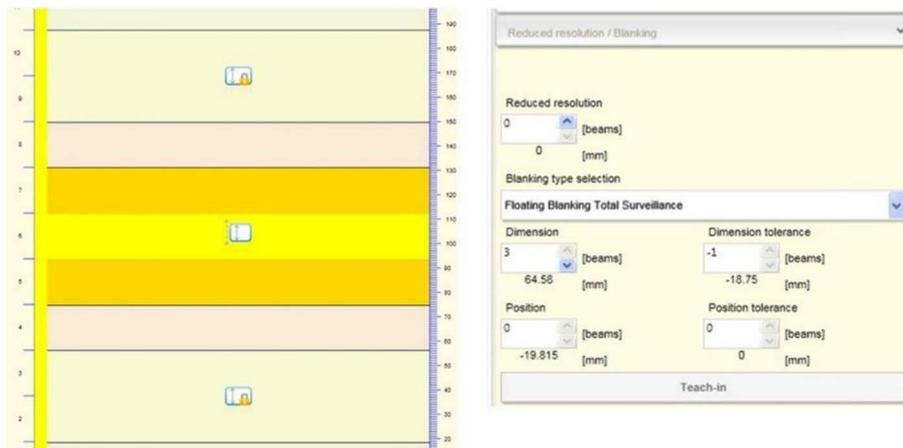
Figure 60 - Floating Blanking with total surveillance
