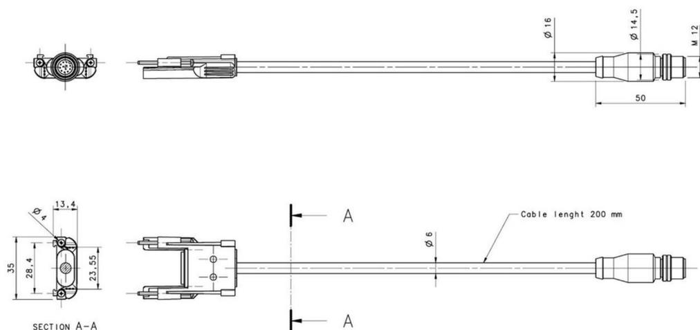
Figure 22 - RX BLANKING - Pigtail cable
