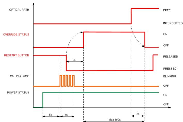
Figure 45 - Startup Override activation and timings
