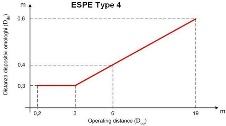
Figure 6 - Minimum distance from reflective surface
