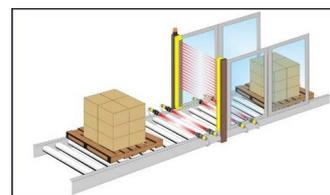
**Figure 18 - Linear version with external Muting sensors**
