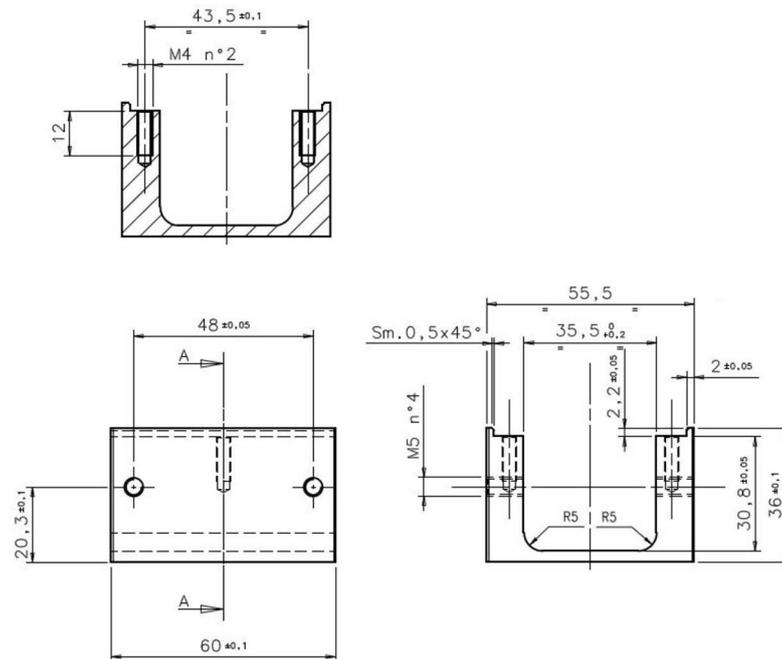
Figure 39 - Mounting bracket
