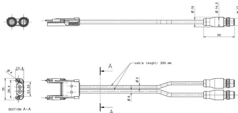
**Figure 23 - RX MUTING - Pigtail cable**
