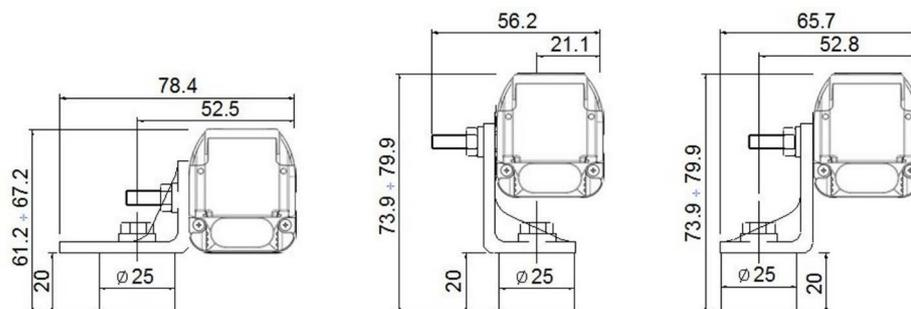
Figure 9 - Angled fixing bracket + Anti-vibration support
