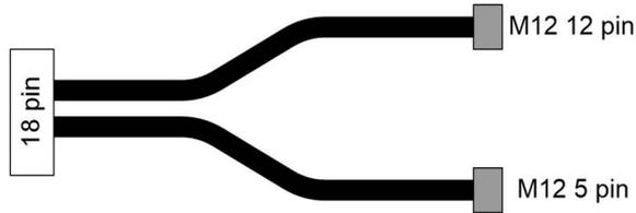
**Figure 2 - Pigtail cable Muting configuration for receiver (CS-R1-75-B-002)**
