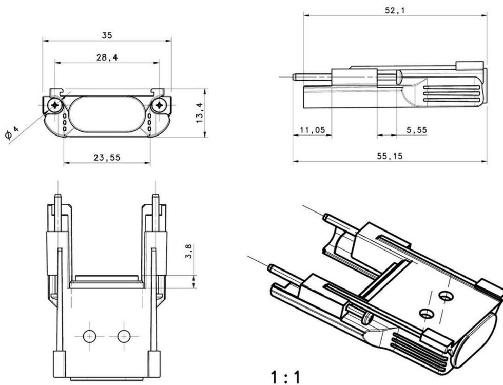
Figure 2 - Dimensions (mm)
