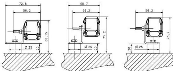
Figure 4 - Angled fixing bracket + Anti-vibration support
