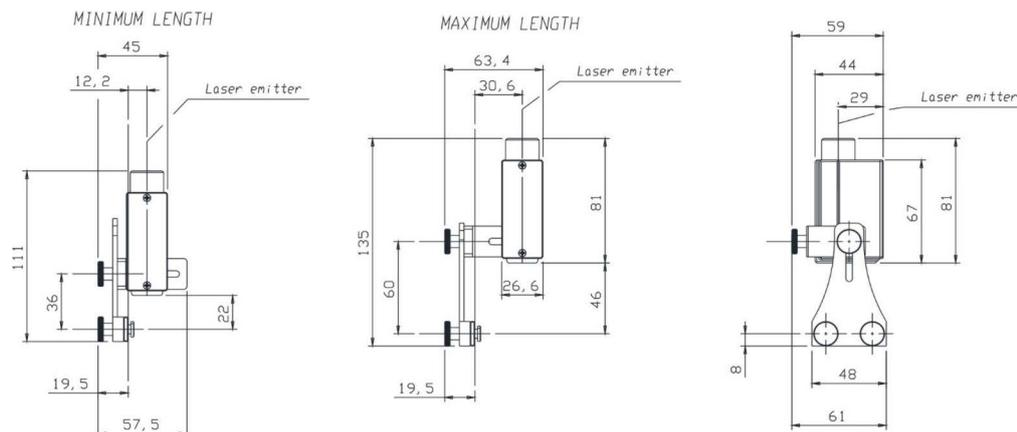
Figure 27 - Dimensions (mm)
