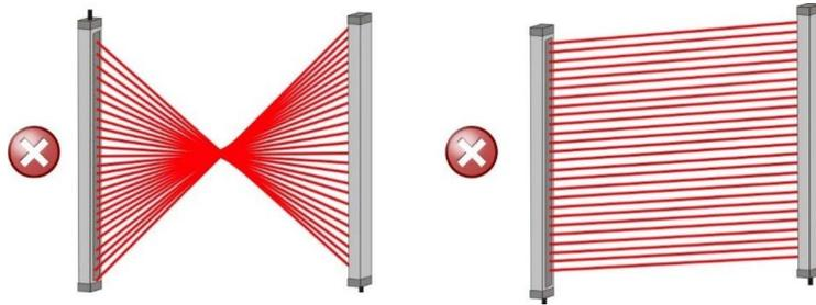
Figure 10 - Wrong light curtain TX-RX orientations
