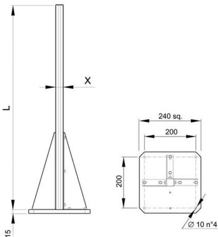
Figure 16 - Dimensions (mm)
