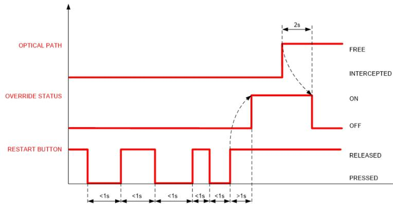
**Figure 46 - Runtime Override activation and timings**
