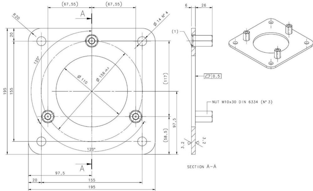
Figure 14 - Dimensions (mm)
