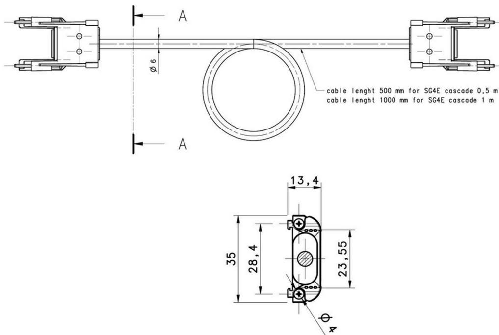
Figure 25 - Dimensions (mm)
