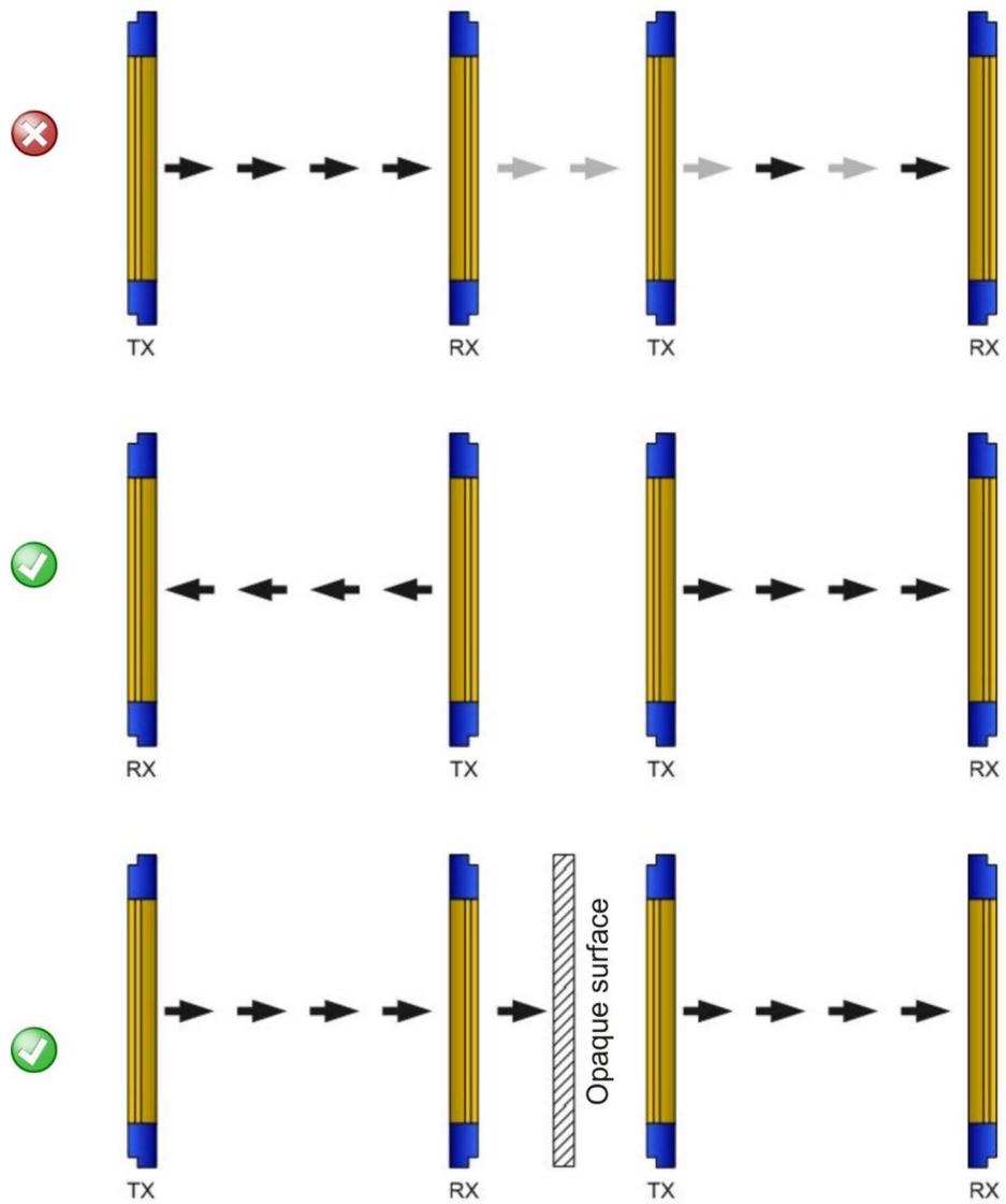
Figure 9 - Recommended positioning for homologous devices
