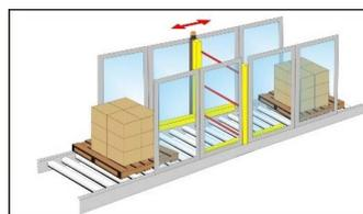
**Figure 17 - T-shaped version with integrated Muting sensors for bidirectional Muting**
