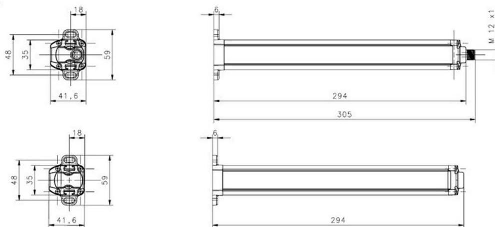
Figure 38 - Dimensions (mm)
