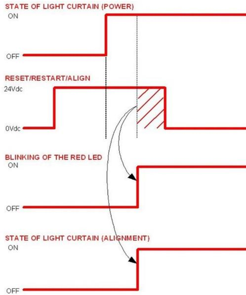
In Alignment Mode ESPE is always in Safe State and the OSSDs are kept OFF.
