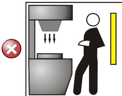
Fig 11 - Wrong light curtain positioning
