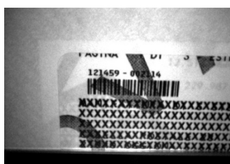
Figure 19 - Overprinted Barcode Readable by Matrix 220 also Through the Envelope Window Film
