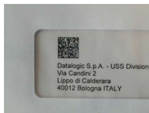
Figure 17 - Address Coded in Data Matrix Symbology for Automated Mail Processing
