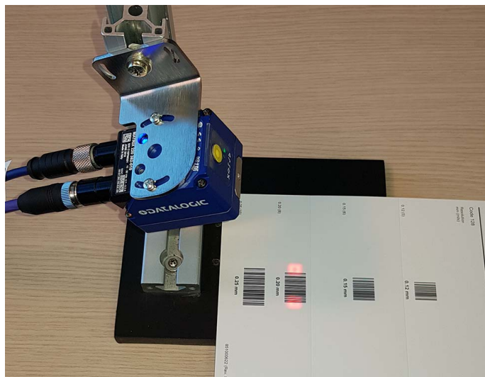
Figure 9 - X-PRESS Interface; Aim/Autofocus Function
