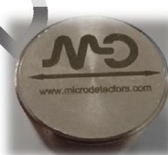
The reference axis of the inclinometer is arranged along the axis of the arrow as shown in the picture.
