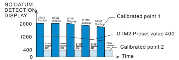
The following sensitivity setting procedure is an example of two point calibration. When there is no workpiece, the intensity of the received light is " 400 ", when there is target, the intensity of light received is " 1000 "
