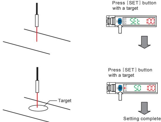
Two point calibration is based on with the target or without the target to calibrate. The preset point is the intermediate value of the above two cases. If the difference between the cases that with or without target is too small, then after the calibration will appear "----" blink for about 2 seconds.
