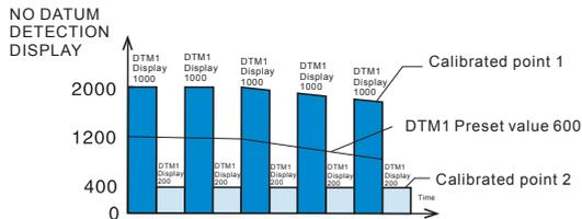
The following sensitivity setting procedure is an example of two point calibration. When there is no workpiece, the intensity of the received light is " 600 ", when there is workpiece, the intensity of light received is " 200 "
