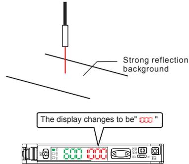
**Notice** If there is no target, the displayed value is lower than " 600 " and after 30 seconds still does not reach " 600 " , please press the [PRESET] button. This will correct the received light intensity to be " 600 " . When the intensity of the received light stops flashing, the correction is completed.
