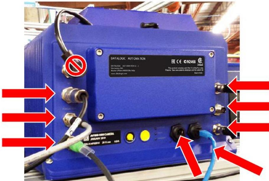
Figure 126: Remove the cables
