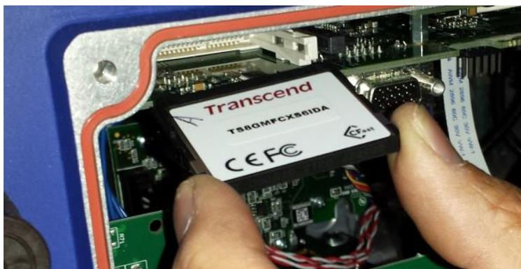
Figure 125: Removing the memory card
