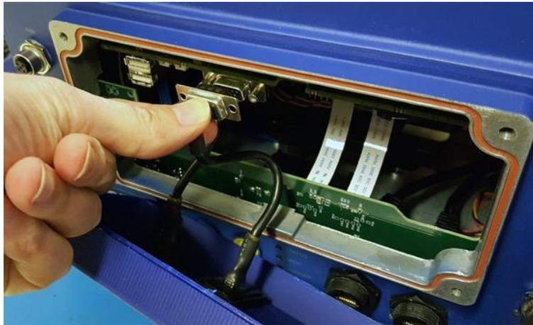
**Figure 91: Connecting VGA Cable**
