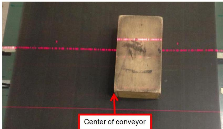
Figure 112: Box of known height placed in RangeFinder scan line
