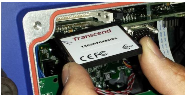
Figure 125: Removing the memory card
