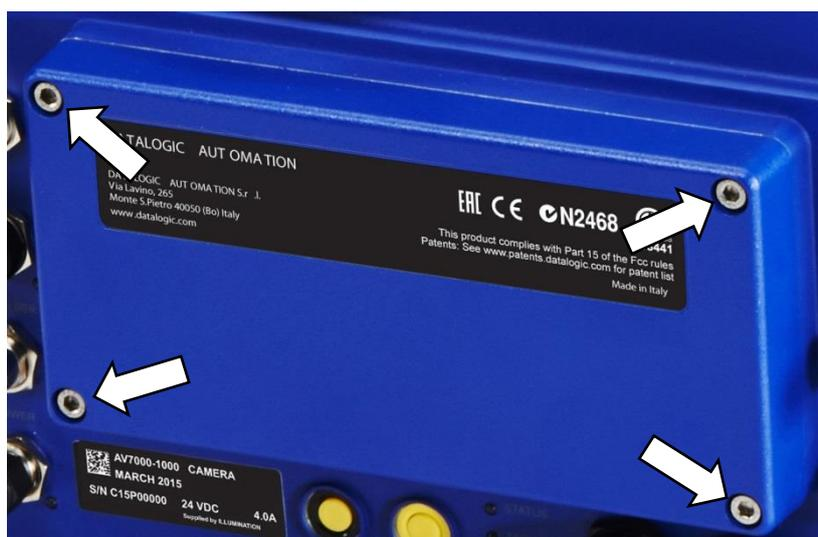
Figure 89: Rear access panel screw locations
