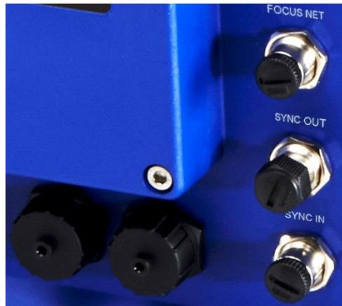
Figure 58: Connector protective caps
