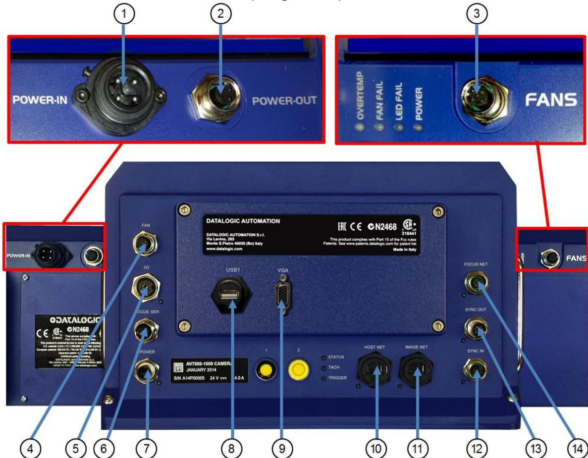
Figure 57: AV7000/AI7000 Connector Panels
