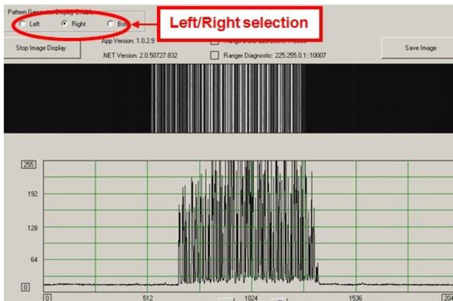
A noticeable discrepancy could indicate a potential problem with the laser diode, and the unit could report erroneous height data.
