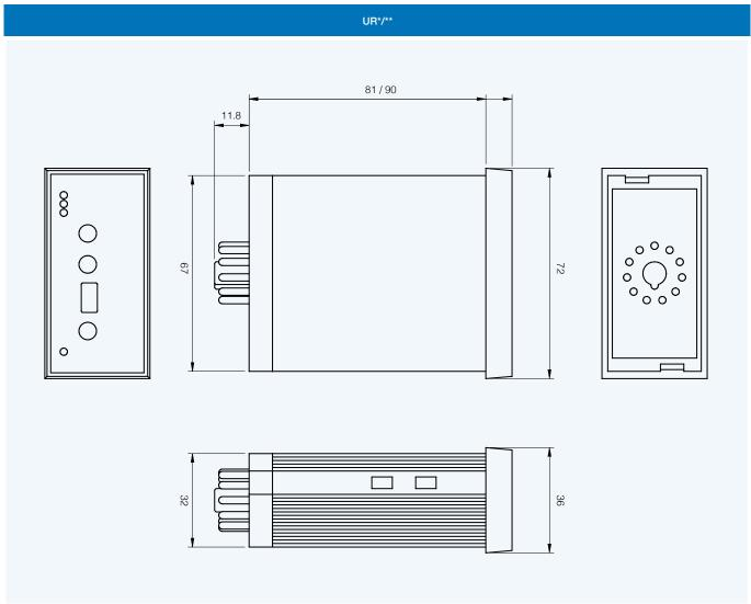
Holes dimensions for mounting on panel: 68x33 mm. Undecal Socket (STZ3) supplied separately.
