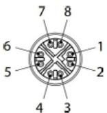
M12 8-pin Standard Ethernet Network Connector Pinout
