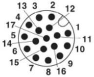
M12 17-pin Power, COM, and I/O Connector Pinout
