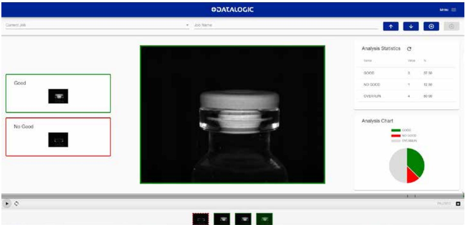
The Smart-VS is provided of a WEB Server User interface for an easy set-up and setting. This is a good option feature when it is needed to setup and change different production jobs depending on variable production format. The information are complete and shown in a clear layout.
