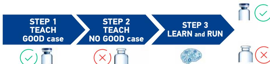
The sensor is especially suited for all the applications where it is needed to solve detection between two well specified object condition classes, like presence or absence of a specific feature or object orientation respect two sides, teaching the sensor with GOOD and NO GOOD condition.
