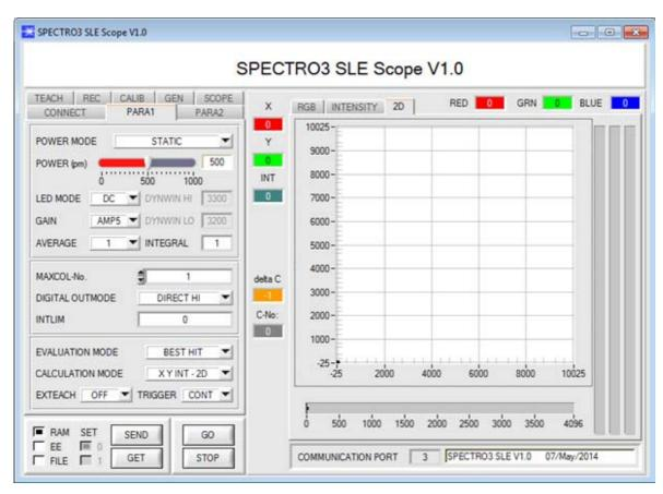
Under Windows® representation of the color value on a PC in numeric form and in a color chart, and representation of RGB values in a time chart. In addition the current RGB values are displayed as a bar chart.
