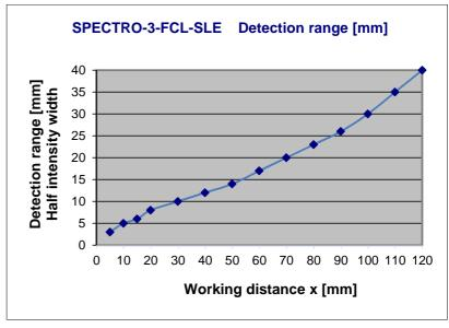
Relative intensity: SPECTRO-3-FCL-SLE: 100% at a working distance of 10 mm (INTENSITY 3785)
