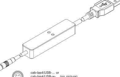
cab-las4/USB-w-... (no picture) (each max. length 5m, outer jacket: PUR)
