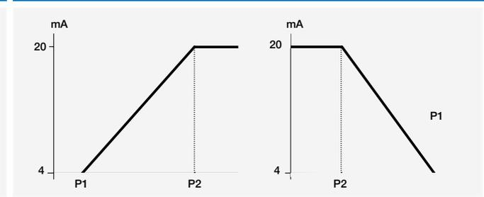
P1 e P2 are the switching points set through the Teach-In cable (pin5). The analogue output is on pin4, linear between P1 e P2. By suitably setting P1 and P2, it is possible to select a positive or negative ramp and the NC or NO status of the output.
