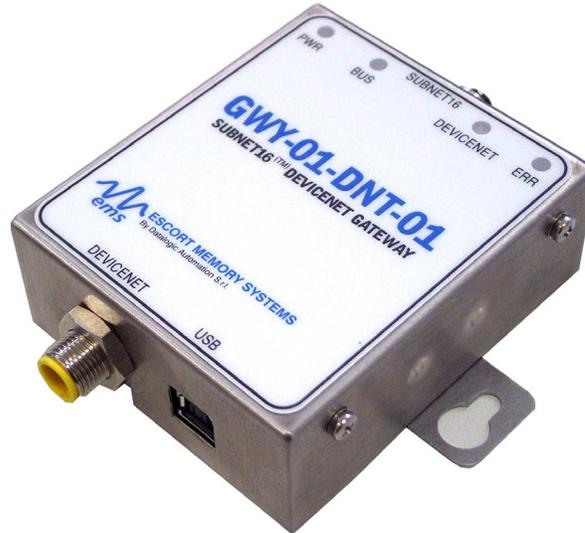
The EMS Gateway supports Subnet 16™, a subnetwork of up to sixteen EMS RFID controller/antenna stations. Subnet16 thus concentrates many read/write devices into one convenient connection point for host networks in the factory or enterprise.
