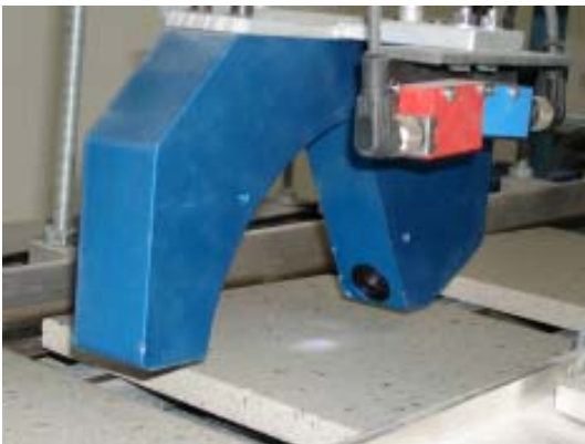
Gloss degree monitoring at plates of stone
