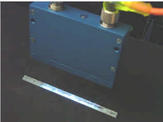
Checking if screw locking varnish was applied
